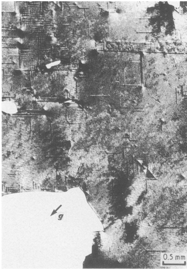
Figure 2 A 00\bar{2} topograph showing the dislocation structure after annealing at 780^\circ\text{C} for 2 h.
